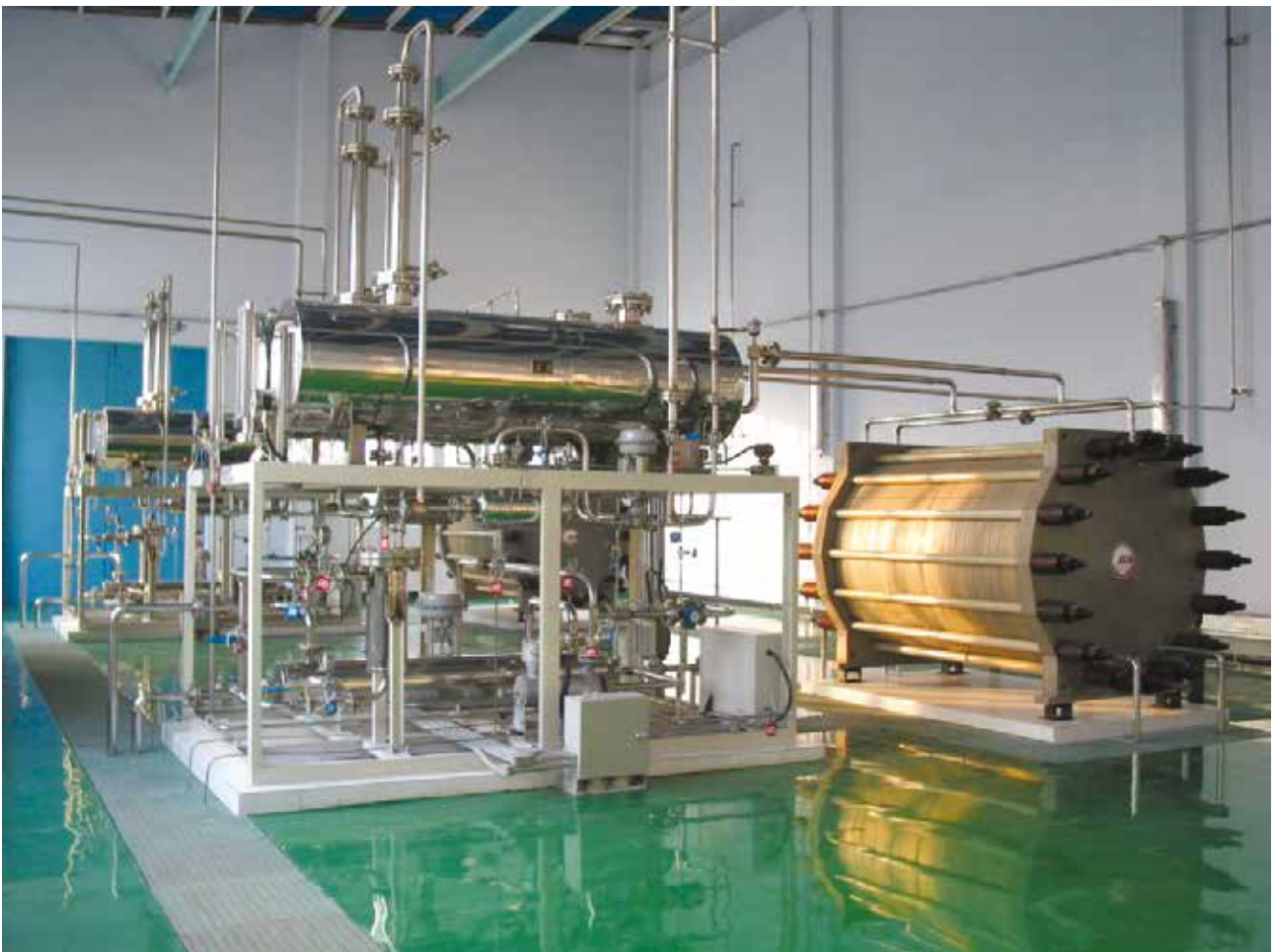
2 electrolyzers and gas separator skids where cooling water enter (and exit) the gas separator from the trench in the floor.
