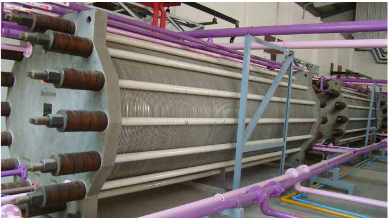
Electrolyzer cellblock where pipes are color marked according to the type of fluid, see next page for the belonging gas separator skid.
