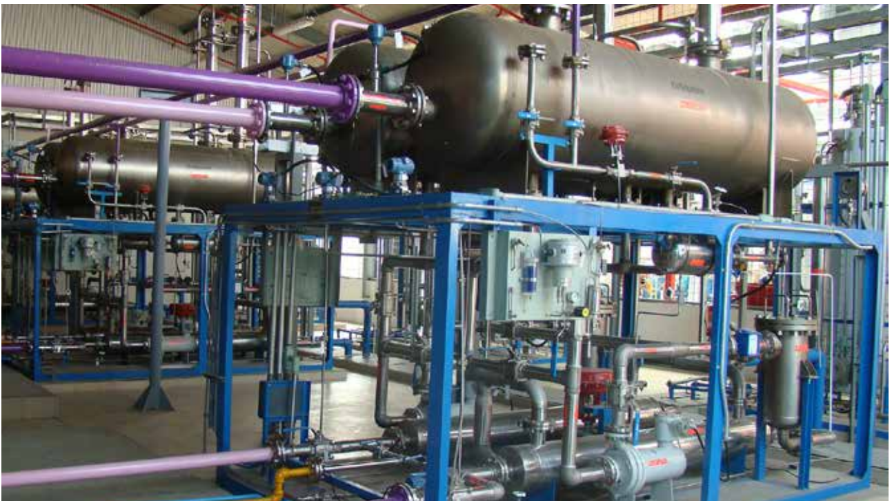
The gas separation skids with lye pumps and coolers.
