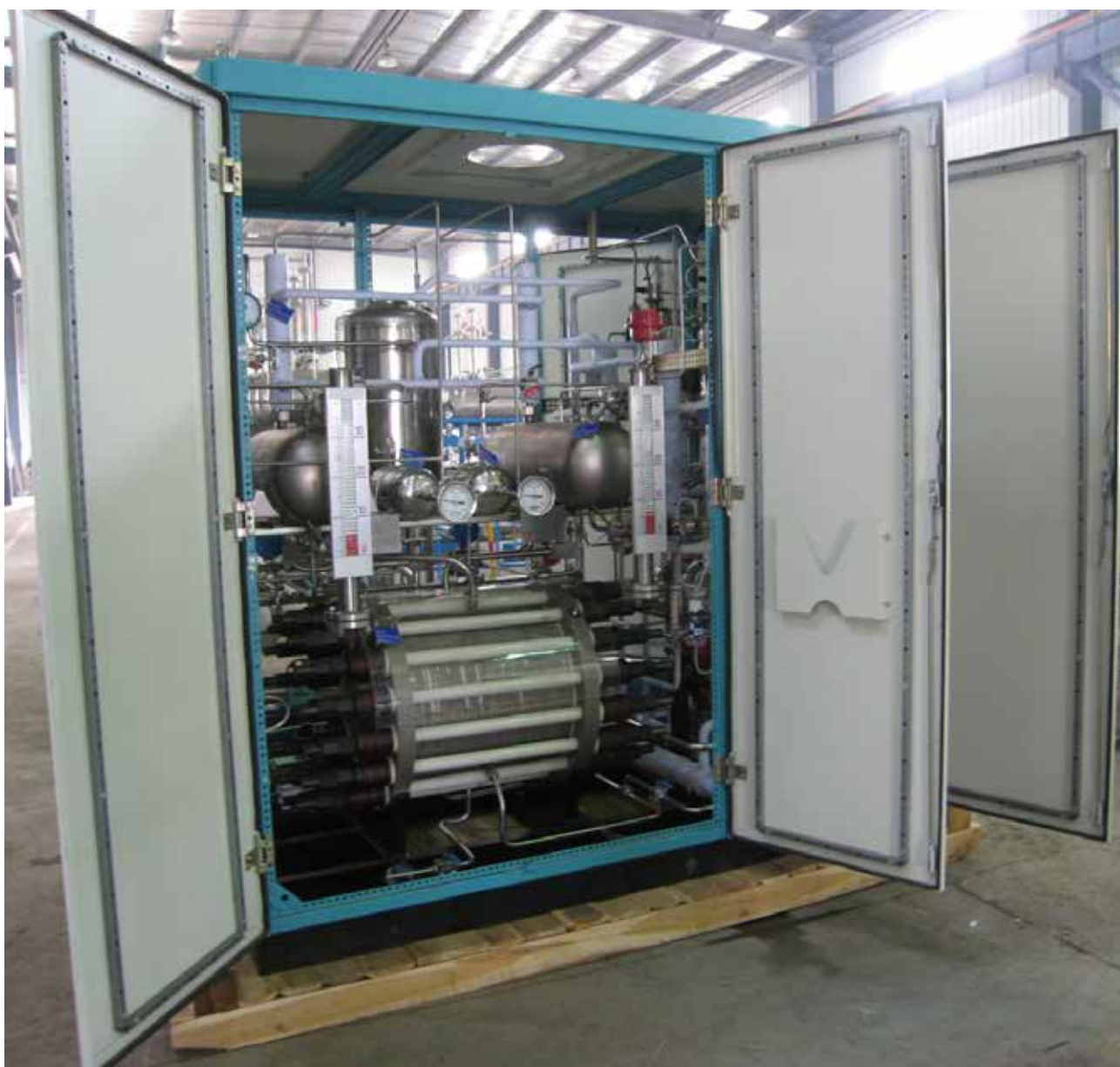
A cabinet mounted compact unit ready to be shipped to customer.
